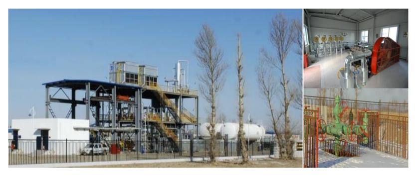
122,000tons of CO<sub>2</sub> were injected and 80,000 tons of CO<sub>2</sub> were storage. 51,000 tons of oil were recovered by May 2010.
