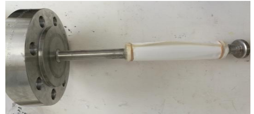
Spiral Wound Module with membrane sample
